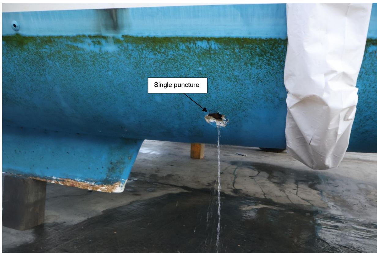
Figure 6: Single puncture observed on the starboard hull
